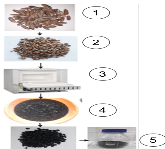
Fig. 1. Different step of Preparation of activated carbon.
